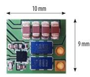
Figure 3: The EPC9093 development board fitted with EPC2053
