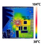
Figure 5: Thermal image of the EPC9093 operating at 500 kHz, 12 V and 20 A with 400 LFM airflow
