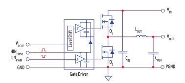
Figure 2: Block diagram schematic of the EPC9093 development board for evaluating 48 V to 5 - 12 V, and 25 A intermediate bus conversion
