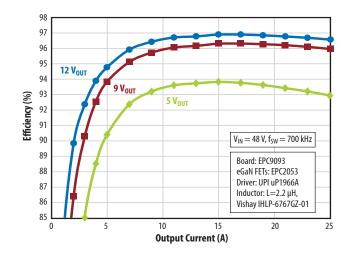
Figure 4: EPC9093 efficiency vs. output current for 48  $V_{IN}$  to 12  $V_{OUT}$ when operating at 700 kHz and using EPC2053 eGAN FETs
