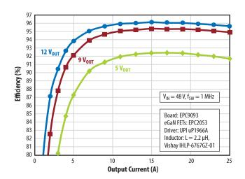
Figure 6: EPC9093 efficiency vs. output current for 48  $V_{IN}$  to 5, 9 and 12  $V_{OUT}$ when operating at 1 MHz and using EPC2053 eGaN FETs
