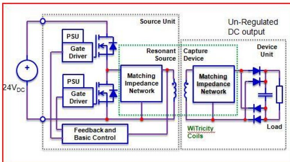
Fig. 1. Wireless power transfer system based on EPC's enhancement-mode gallium nitride (eGaN) FETs. The power converter implemented in this system is a class D power amplifier operating at 6.78 MHz.
