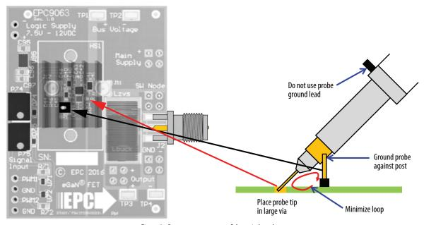
Figure 3: Proper measurement of the switch nodes
