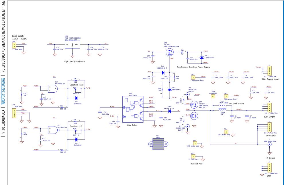
Figure 7: EPC9063 Schematic
