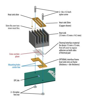
Figure 6: Assembly of the heatsink kit
