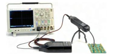
Figure 4: Tektronix IsoVu measurement setup.
