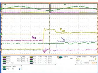
Figure 5: Upper gate and lower gate measurements using the Tektronix IsoVu and switch-node voltage measurement using the TPP1000 probe.
