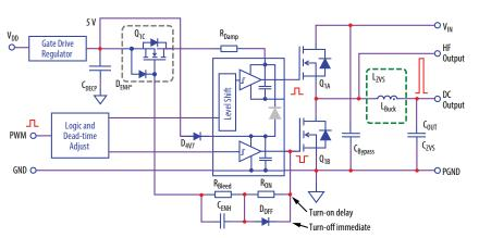
Figure 1: Block diagram of EPC9063 development board
