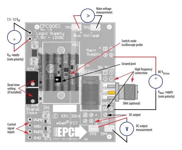
Figure 2: Proper connection and measurement setup
