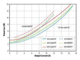
Figure 5: Power loss comparison between eighth brick converters
