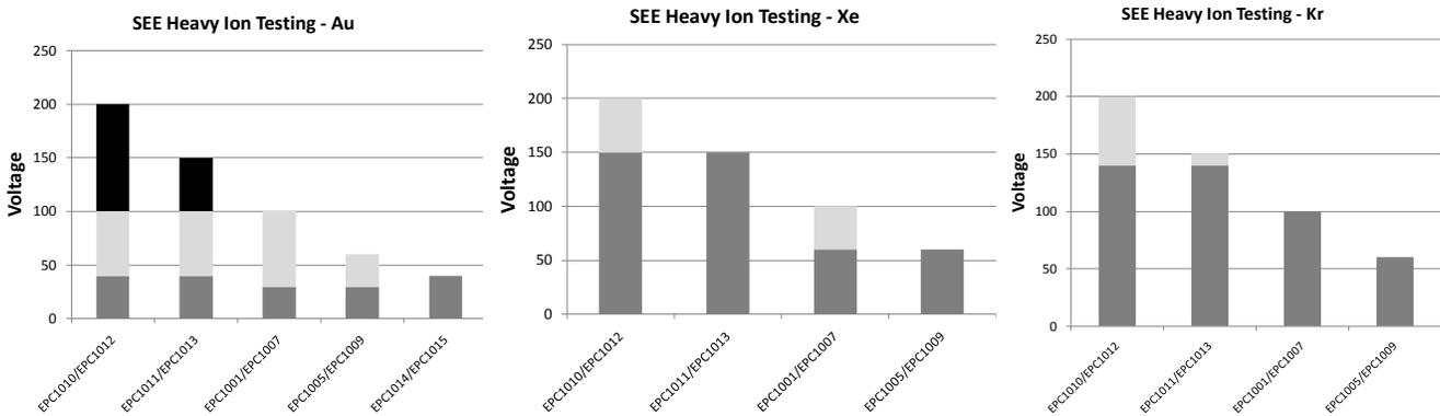
**Figure 2.** SEE Results for Au, Kr, and Xe bombardment. Dark grey bars represent the voltage range within which devices remained inside data sheet limits. Light grey bars represent the range where devices continued to function but drain-source leakage exceeded data sheet. Black bars represent regions where devices catastrophically failed
