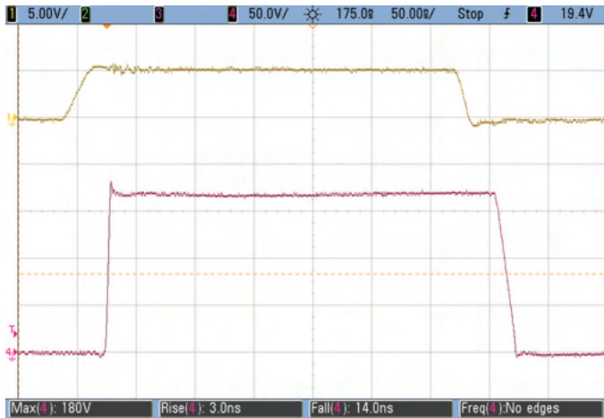
Figure 4: Waveforms for V_{IN} = 170\text{V} to 5\text{V}/5\text{A} (100kHz) Buck converter CH1: V_{PWM} Input voltage – CH4: ( V_{OUT} ) Switch node voltage
