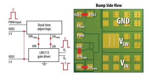
Figure 2: Single PWM input setup.
