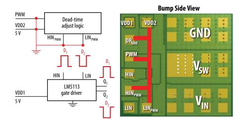
Figure 3: Two PWM input setup.
