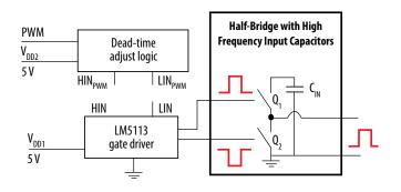
Figure 1: Block diagram of EPC9201/3 development board.
