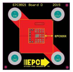
Figure 8: Top layer without filled thermal vias.
