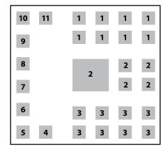
Pin 1: Input Voltage, V<sub>IN</sub> Pin 2: Switching Node, V<sub>SW</sub> Pin 3: Power Ground, P<sub>GND</sub> Pin 4: Driver Voltage, V<sub>DD2</sub> Pin 5: Driver Voltage, V<sub>DD1</sub> Pin 6: Driver Ground, DR<sub>GND</sub> Pin 7: PWM Input, PWM Pin 8: High Side Input, HIN Pin 9: PWM High Side Input, HIN<sub>PWN</sub> Pin 10: Low Side Input, LIN
