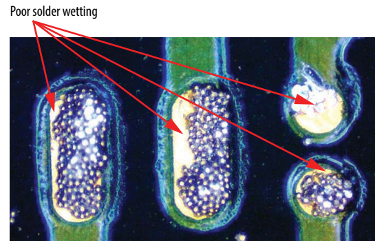
Figure 16: Example of poor solder wetting.
