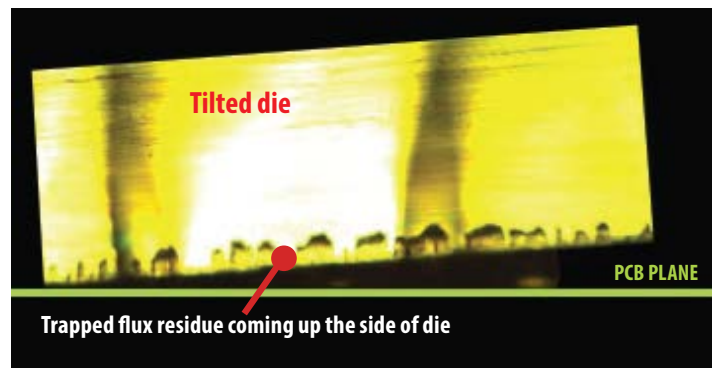
Figure 19: Side view of an eGaN device with severe die tilt after soldering.
