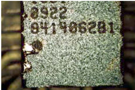
Fig 4c: EPC1001 part (above) passed 1000 Cycle TC -40°C to 125°C. Die width ~1900 μm Back side chip >250 μm
