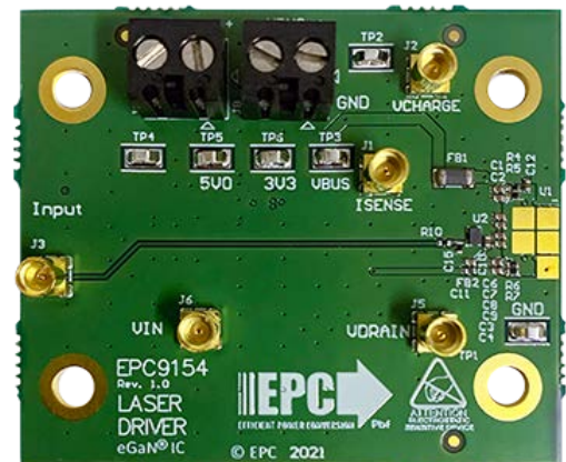
EPC9154 Short Range Lidar 10 A laser pulse peak 410 ps on time, 320 ps off time
