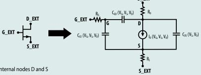
Figure 5: EPC's GaN model The nonlinear capacitors and current sources are combined to produce the time dependent electrical behavior of the device. A device circuit schematic is shown in Figure 5. The main components are the voltage controlled current source, ID, Non-linear capacitors,  $C_{GD}$ ,  $C_{GS}$ , and  $C_{SD}$ , and input resistors  $R_S$ ,  $R_D$ , and R<sub>G</sub>.
