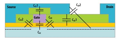
Figure 4: Schematic of capacitance sources
