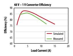
Figure 13: Comparison of simulated and measured efficiency for 48 V - 1 V converter.
