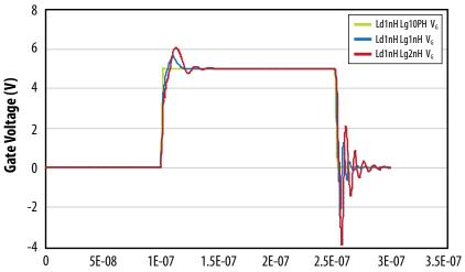
Figure 7: A) Comparison of drain node oscillations vs different stray inductance levels. B) gate node oscillations vs stray gate inductance.
