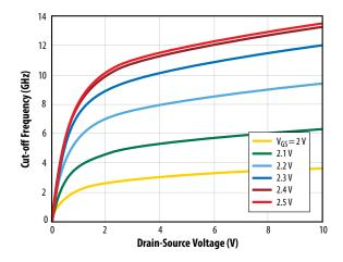
Figure 15: (Left) Simulated cut-off frequency versus  $V_{GS}$  for  $V_{DS} = 1,2,3,4,5,6$  V; (Right) Cut-off frequency versus  $V_{DS}$  for  $V_{GS} = 2.0-2.5$  V (EPC2015)
