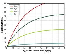
Figure 2: Transfer and output curves for EPC1001 device model
