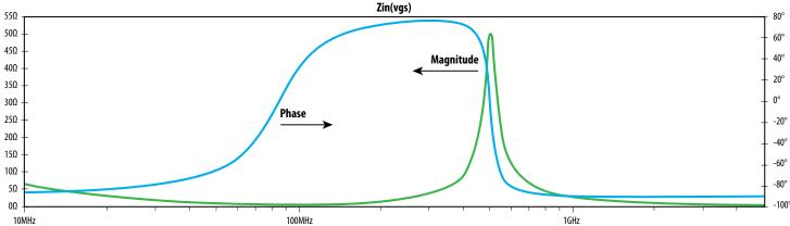
Figure 16: (Top Left) Circuit schematic for gate impedance matching simulation. (Bottom) Input impedance (magnitude and phase) versus frequency looking into gate with matching network tuned for 500 MHz. (Top Right) Smith chart of gate input impedance, both with and without matching network.
