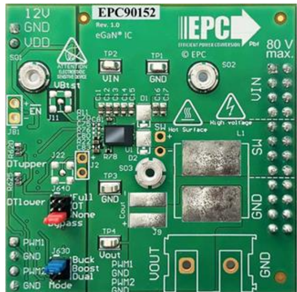
Figure 7: EPC90152 Evaluation Board (see EPC90152 Quick Start Guide for details)
