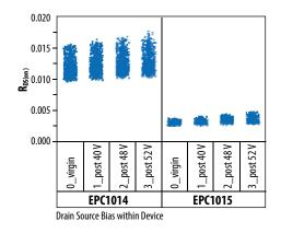
Figure 6: The R<sub>DS(on)</sub> values post various drain biases are shown for EPC1014 and EPC1015, the two 40 V products.
