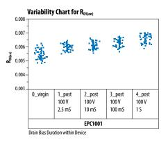
Figure 5: R<sub>DS(on)</sub> values after 100 V bias for various durations.
