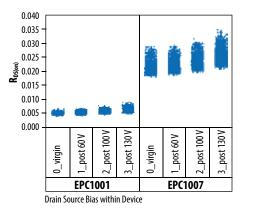
Figure 7: The R<sub>DS(on)</sub> values post various drain biases are shown for EPC1001 and EPC1007, the two 100 V products.
