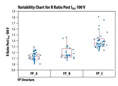
Figure 4: Field plate has big impact on dynamic  $R_{DS(on)}$ . An example is shown comparing field-plate structure A, B, and C that were studied during product development.
