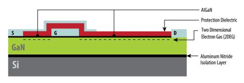
Figure 1: GaN on silicon devices have a very simple structure similar to a lateral DMOS device and are built in a standard CMOS foundry
