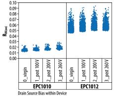
Figure 8: The R<sub>DS(on)</sub> values post various drain biases are shown for EPC1010 and EPC1012, the two 200 V products.
