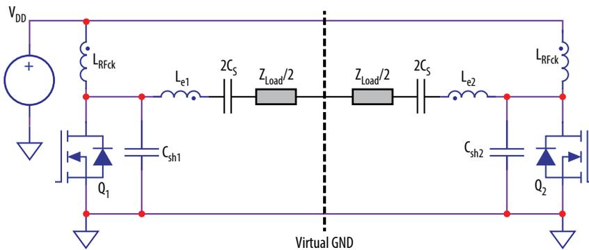
Figure 5. Half-circuit analysis of a differential class E amplifier
