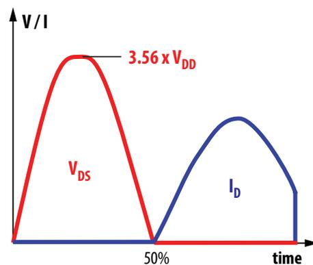
Figure 3. Ideal FET voltage and current waveforms for the class E amplifier
