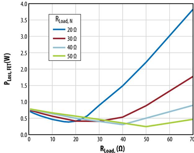
Figure 7. Simulated FET losses for a range of  $R_{Load}$  in the differential class E amplifier with different nominal  $R_{Load,N}$
