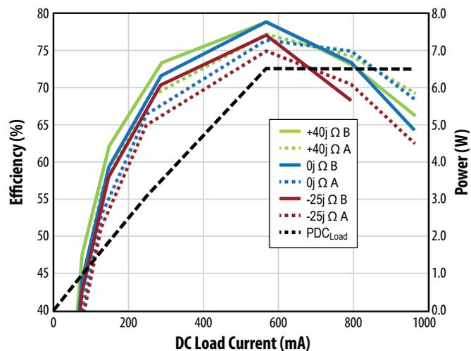
Figure 12. Total system efficiency comparison between two possible device coil orientations
