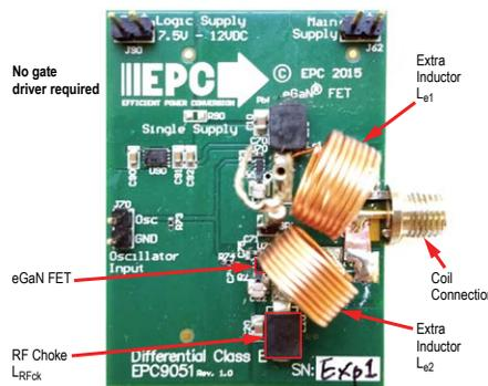
Figure 8. Differential-mode class E configured EPC9051 development board
