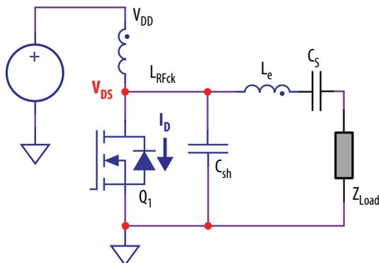
Figure 2. Schematic of a single-ended class E amplifier
