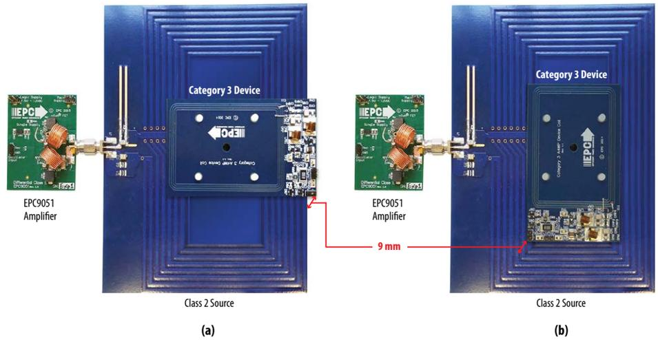
Figure 10. System test setup for wireless power transfer: differential class E amplifier (EPC9051) with class 2 source coil and category 3 device coil. Two possible device coil orientations.
