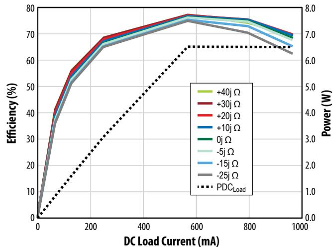
Figure 11. Measured total system efficiency with a category 3 device. Orientation A
