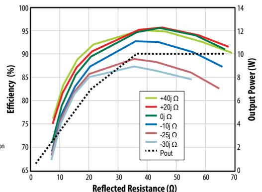
Figure 9. Measured total amplifier efficiency including gate driver losses over the whole required impedance range
