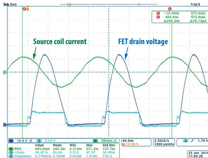
Figure 13. Source coil current and FET drain voltage waveform of the differential class E amplifier. Operation conditions: device coil orientation A, source coil tuned to  $+20j\Omega$ , 16.3 V input,  $10\Omega$  DC load, 6.5 W DC output power, and 75% total system efficiency.
