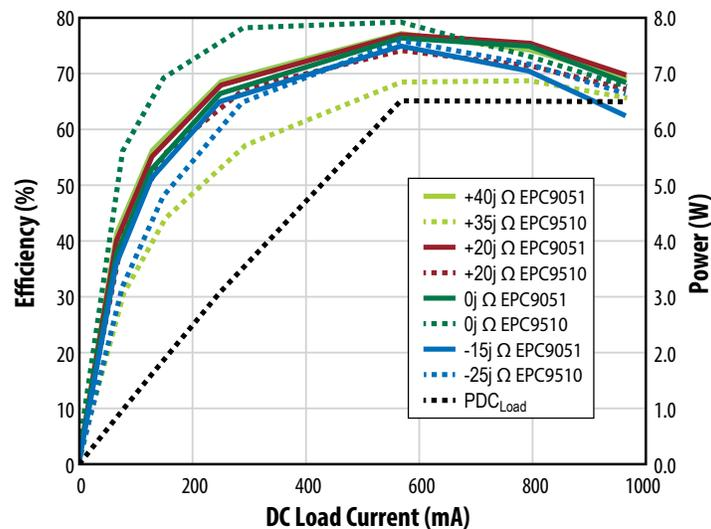
Figure 14. Efficiency comparison of differential class E and ZVS class D amplifiers in wireless power systems.
