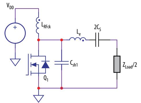
Figure 6. Equivalent circuit for designing a differential class E amplifier
