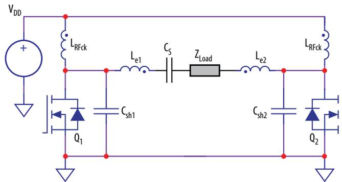
Figure 4. Schematic of a differential class E amplifier
