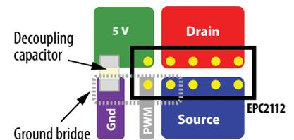
Figure 5. Example layout with low power loop inductance.
