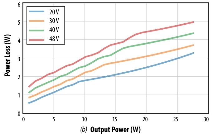
Figure 6. Measured (a) total efficiency and (b) total power loss for EPC9131 SEPIC converter using EPC2112 for various input voltages delivering 19 V output over the load range from 1 W through 27 W.
