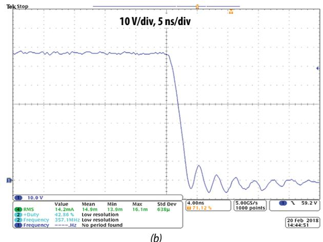
Figure 7. Switch-node voltage waveforms of the SEPIC at 48V input, 19V and 27 W output. (a) rising edge and (b) falling edge.
