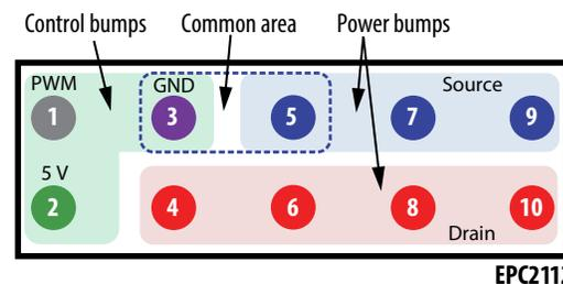
Figure 4. Bump assignment for easy layout.
