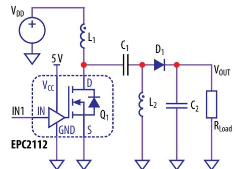
Figure 2. Schematic of SEPIC using EPC2112 with integrated gate driver.
