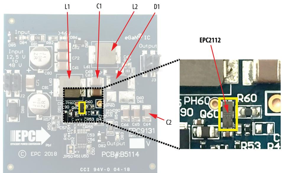
Figure 3. Photo of EPC9131 SEPIC regulator with EPC2112.
