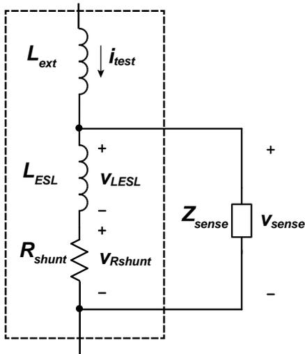
Figure 23. Current measurement shunt resistor with parasitic inductance.
