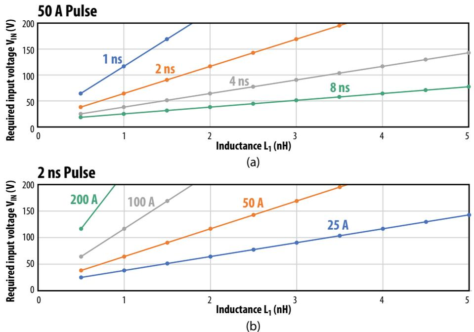
Figure 9. Bus voltage  $V_{IN}$  versus inductance  $L_1$ . (a) shows effect of pulse width for a specific peak pulse current of 50 A, and (b) shows the effect of current for a specific pulse width of 2 ns FWHM.
