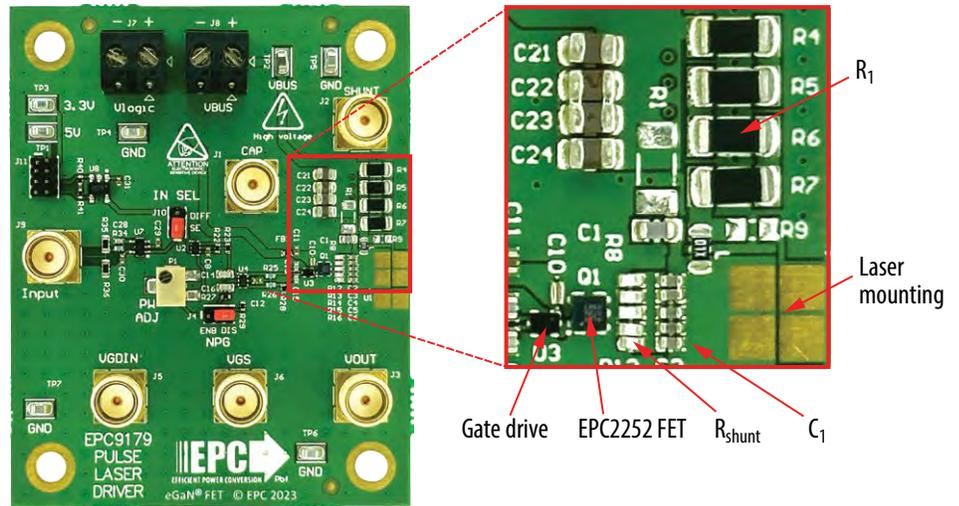
Figure 16. EPC9179 resonant pulse driver with closeup of power loop that highlights the key components of the resonant network. Inductance  $L_1$  is not shown because it is strictly due to stray inductance of the power loop components and the PCB.
