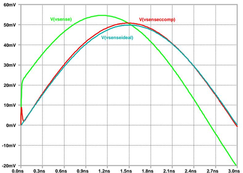
Figure 24. Simulation of current shunts and comparison of results for ideal shunt, uncompensated shunt with ESL, and compensated shunt using RC network. In this simulation,  $R_{shunt} = 100 \text{ m}\Omega$  and  $L_{shunt} = L_{ESL} = 40 \text{ pH}$ . A half-sine pulse with pulse width of 2 ns FWHM.
