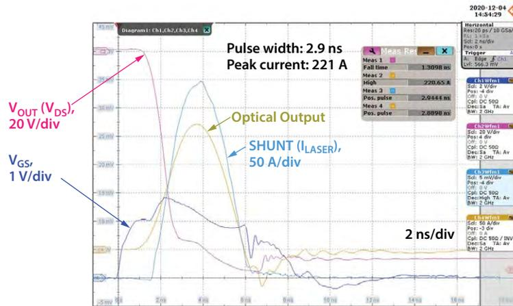
Figure 21. Waveforms for the EPC9150 demo board using an ams OSRAM SPL S4L90A\_3 A01 four channel triple laser diode mounted with the EPC9989 interposer. All channels are connected in parallel.  $V_{BUS} = 150$  V.
