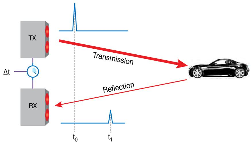
Figure 2. Simplified operation of DToF lidar system
