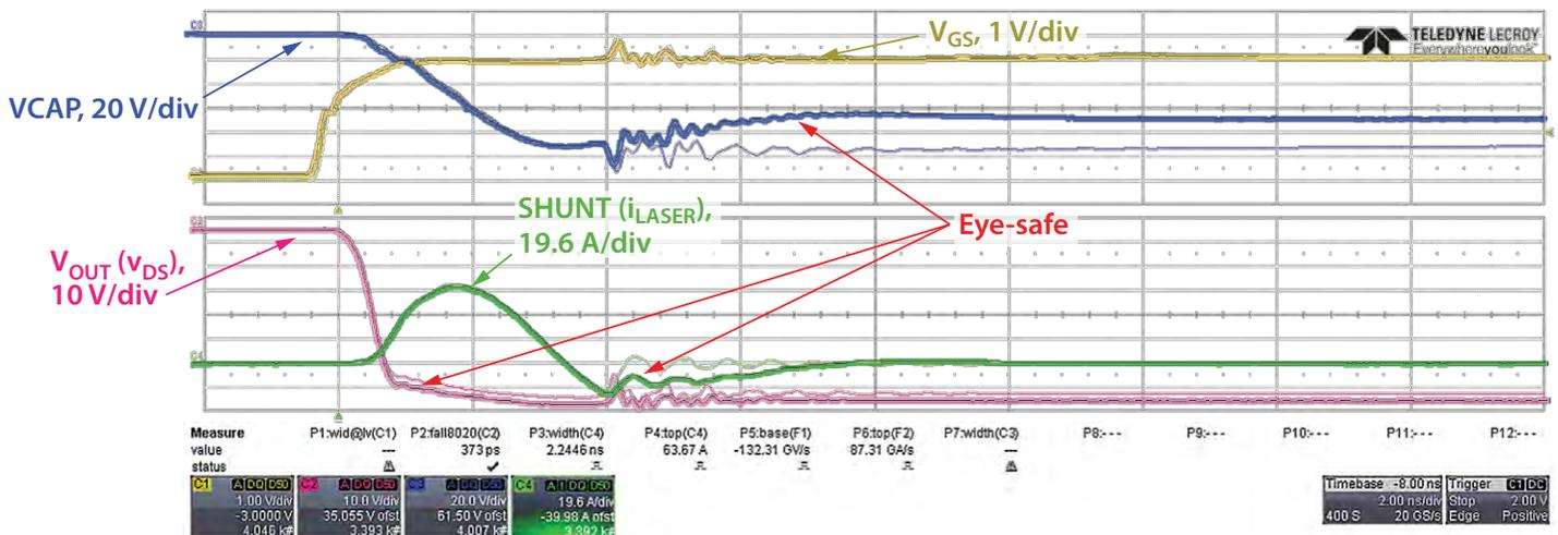
Figure 27. Comparison of conventional and fail-safe charging modes for an EPC9179 evaluation board with an ams OSRAM S1L90A\_3 A01 laser installed. The thin traces show the unmodified board and the thick traces show the results with the fail-safe modification.
