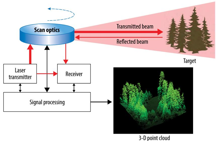
Figure 1. Basic lidar system
