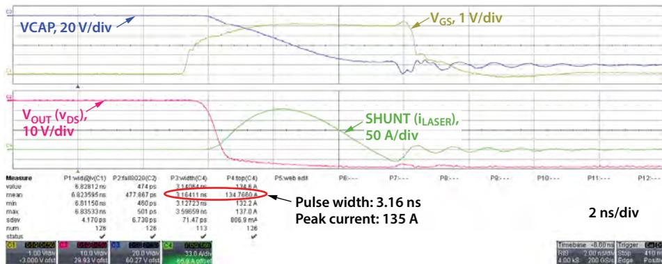
Figure 20. Waveforms for the EPC9181 demo board using an ams OSRAM SPL S4L90A\_3 A01 four channel triple laser diode mounted with the EPC9989 interposer. All channels are connected in parallel.  $v_{BUS} = 70$  V.
