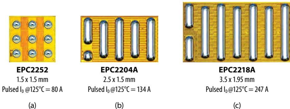
Figure 10. EPC2252 (a), EPC2204A (b), and EPC2218A (c) 80 V eGaN FETs, to scale [12]. Each of these FETs uses a chip-scale package for extremely low inductance and are automotive qualified according to the AEC-Q101 standard.
