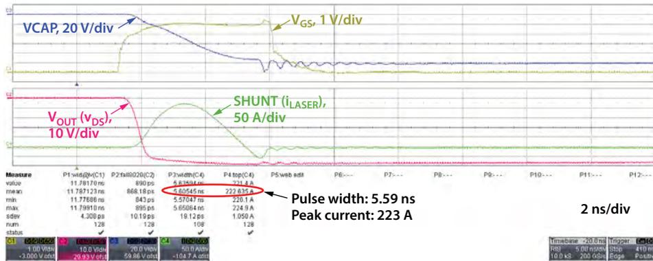
Figure 19. Waveforms for the EPC9180 demo board using an ams OSRAM SPL S4L90A\_3 A01 four channel triple laser diode mounted with the EPC9989 interposer. All channels are connected in parallel.  $v_{BUS} = 70$  V.
