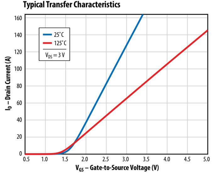
Figure 6 - Transfer curves for EPC2619
