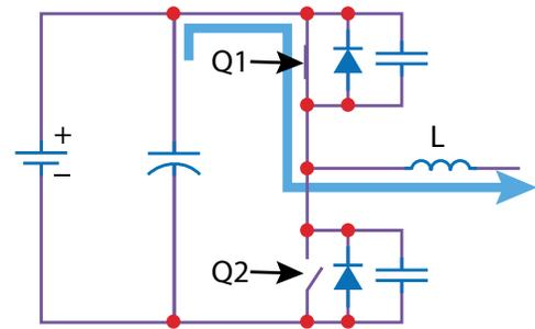
Figure 1 - Hard switched half bridge
