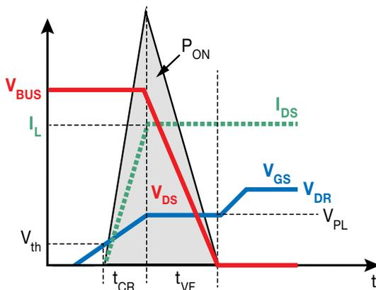
Figure 2 - Turn on simplified waveform
