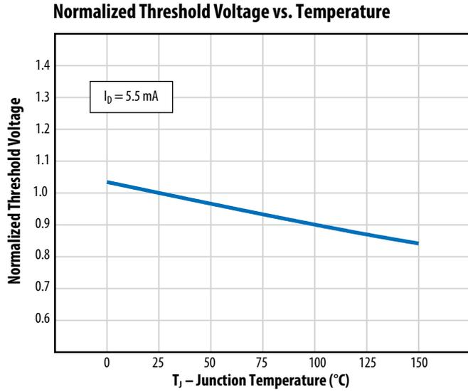
Figure 5 -  $V_{th}$  vs.  $T_J$  for EPC2619
