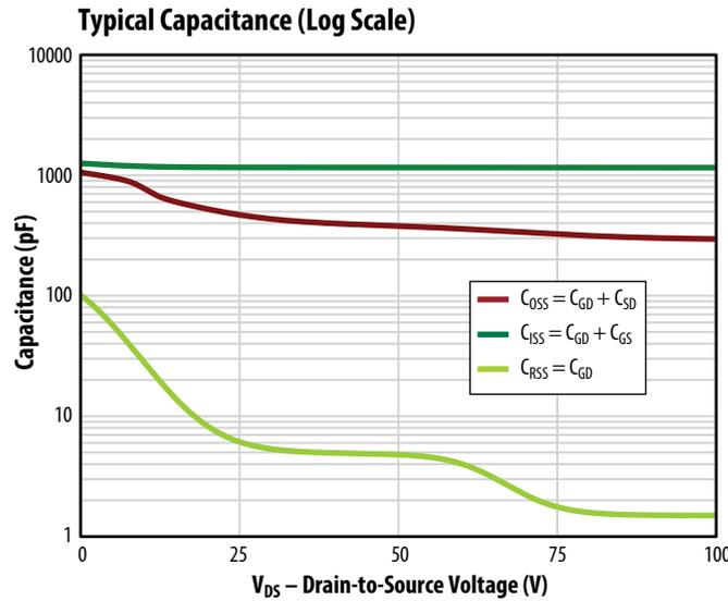
Figure 7 - Capacitance curves from EPC2619
