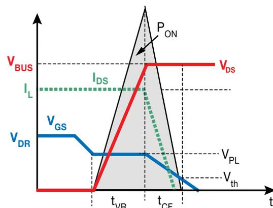
Figure 3 - Turn off simplified waveform
