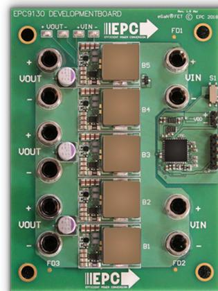
Figure 7: EPC9130 five-phase board with 12 A per phase has a maximum output current of 60 amps, making the board capable of over 700 W
