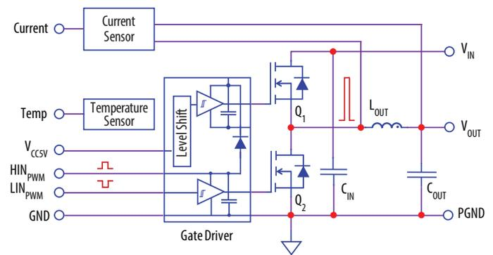
Figure 3. Block diagram schematic of the EPC9205 development board, fitted with EPC2045, is ideal for 48 V to 5 - 12 V intermediate bus conversion
