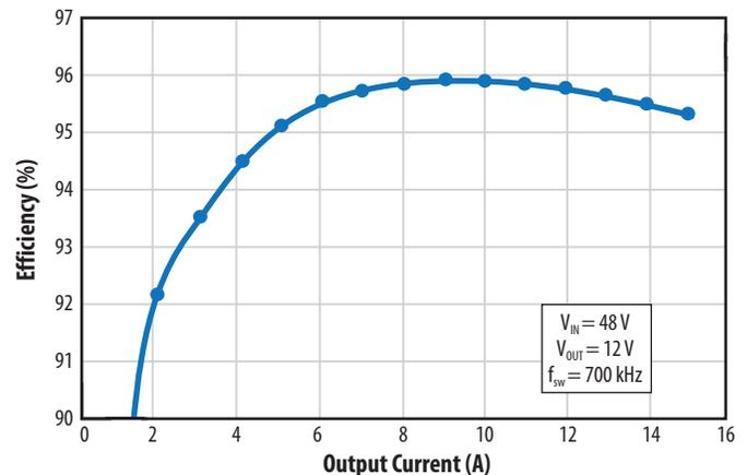
Figure 4. EPC9205 efficiency vs. output current for 48 V<sub>IN</sub> to 12 V<sub>OUT</sub> when operating at 700 kHz and using EPC2045 eGaN FETs
