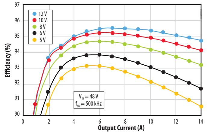
Figure 5. EPC9205 efficiency vs. output current for 48 V<sub>IN</sub> to 5 - 12 V<sub>OUT</sub> when operating at 500 kHz and using EPC2045 eGaN FETs
