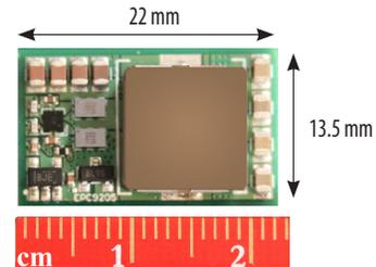
Figure 2: EPC9205 development board boasts a power density of 1400 W/in<sup>3</sup> when operating at 48 V input, 12 V output at 10 A load
