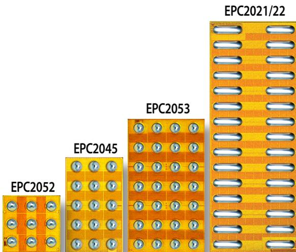
Figure 6: GaN power modules for DC-DC conversion, increasing efficiency across the 48 V to point-of-load power architecture
