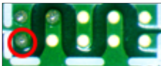
Figure 2: Correct application of solder to a pad
