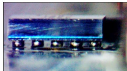
Figure 5: Correctly seated die showing well rounded bumps and no flux residue between the bumps
