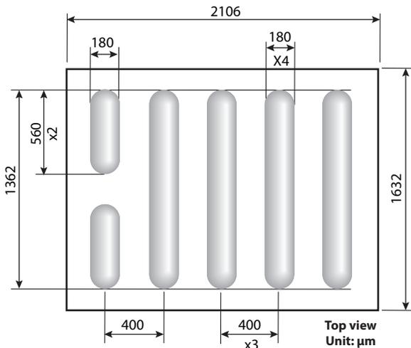
Solder mask thickness recommendation is 25 µm (1mil) or less
