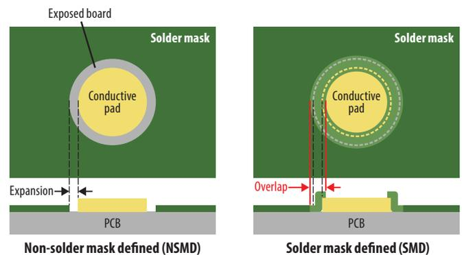
Figure 2. Land Pad comparison: NSMD (Not recommended) vs SMD (Recommended)
