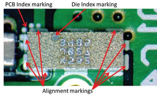
Figure 4. Example of proper silkscreen design
