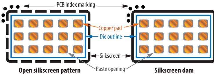
Figure 3. Pad design with silkscreen comparison
