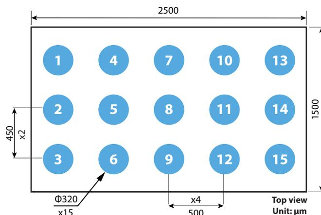
Solder mask thickness recommendation is 25 µm (1mil) or less.
