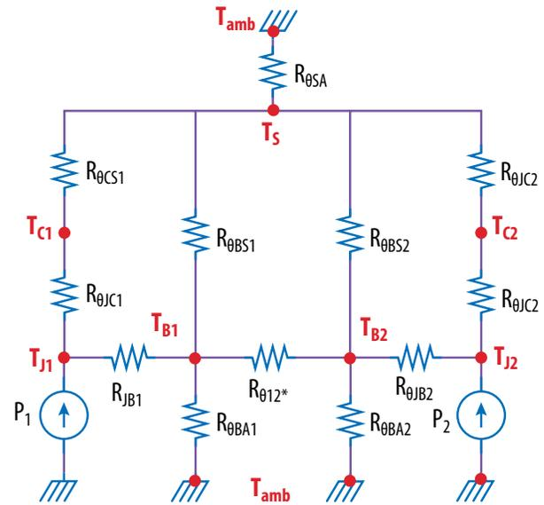
Figure 9: Thermal resistance circuit model with heat sink attachment and corresponding cross-sectional image. Note:  $T_s$  assumed uniform in location of FETs.
