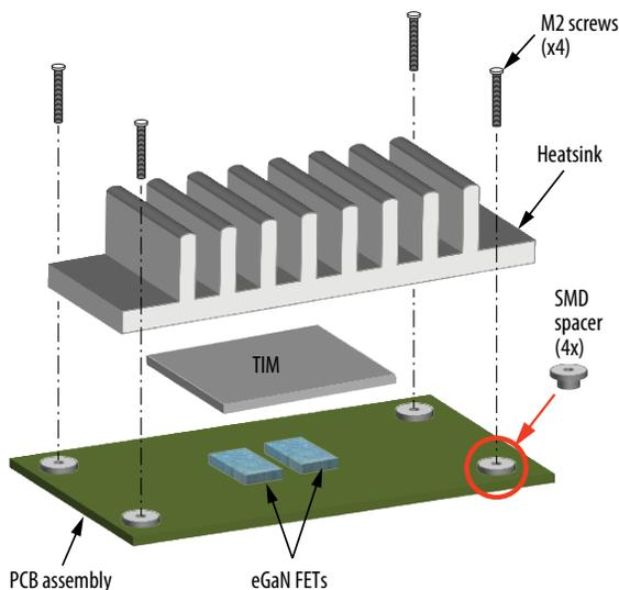
Figure 5: An example of heatsink assembly using screws.
