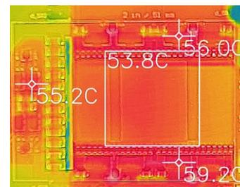
Figure 6: Thermal image of the LLC converter operating at 54 V input and 900 W load
