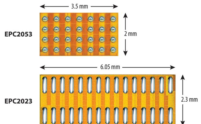
Figure 2: Photo of the bump side of EPC2053 (top) and EPC2023 (bottom)
