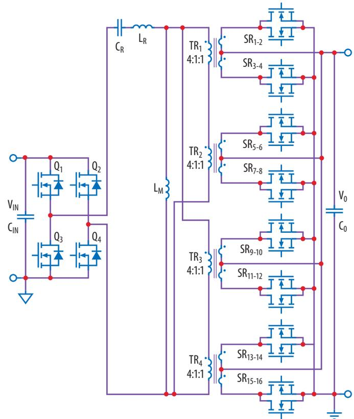
Figure 1: Power architecture schematic of the 900 W, 48 V to 6 V LLC converter
