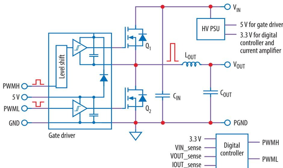
Figure 1. Simplified schematic of the eGaN FET-based synchronous buck converter
