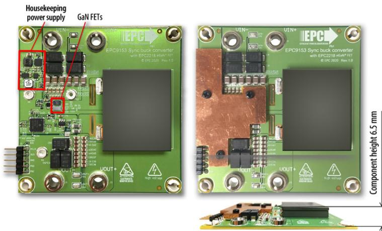
Figure 4. Photo of the 56 V to 20 V, 250 W synchronous buck converter EPC9153 without (left) and with (right) the heat-spreader installed
