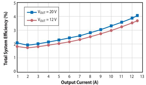
Figure 7. Total system efficiency including the housekeeping power consumption at 48 V input and different output voltages
