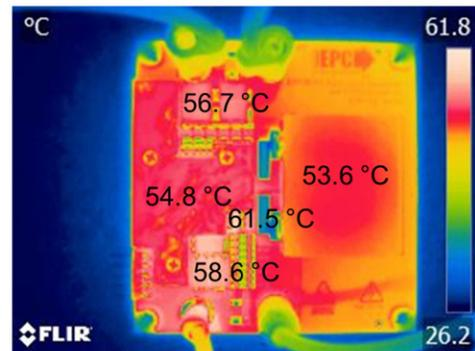
Figure 8. Thermal image of the synchronous buck converter operating at 56 V to 20 V and 12.5 A output and thermal steady state with the heat-spreader and without forced air
