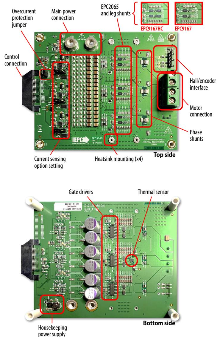
Figure 1. Photo overview of the **EPC9167** **EPC9167HC** board highlighting the main sections.
