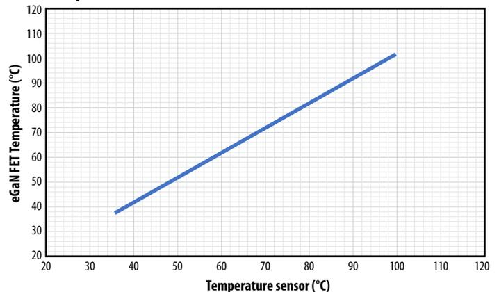
Figure 5. eGaN FET case temperature vs. temperature sensor placed on bottom of the PCB. Operation under natural convection without heatsink.
