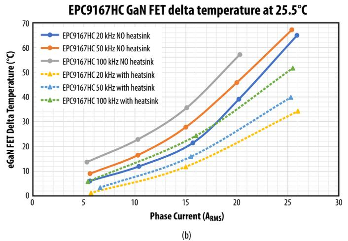
Figure 7. EPC9167 (a) and EPC9167HC (b) GaN FET temperature (\*) increase vs. the ambient temperature [25.5°C]. Measurements taken at various PWM frequencies. (\*) With heatsink, junction temperature has not measured directly. The indicated delta temperature with heat sink is the hottest point at the base of the heat sink.
