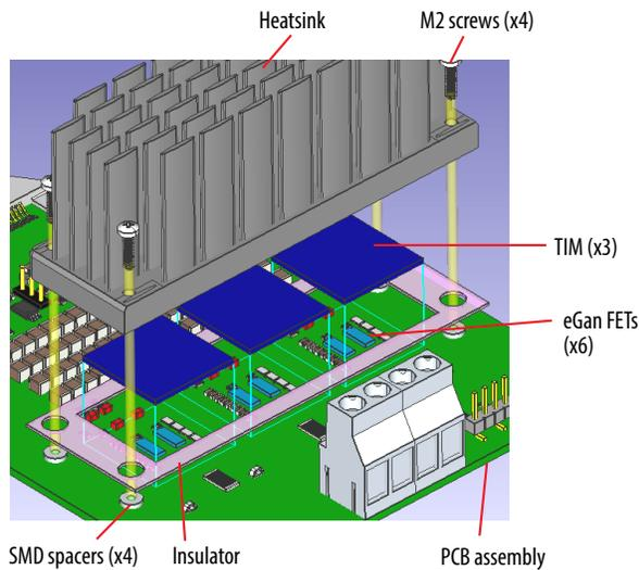
Figure 2. Details for attaching a heatsink to the board.
