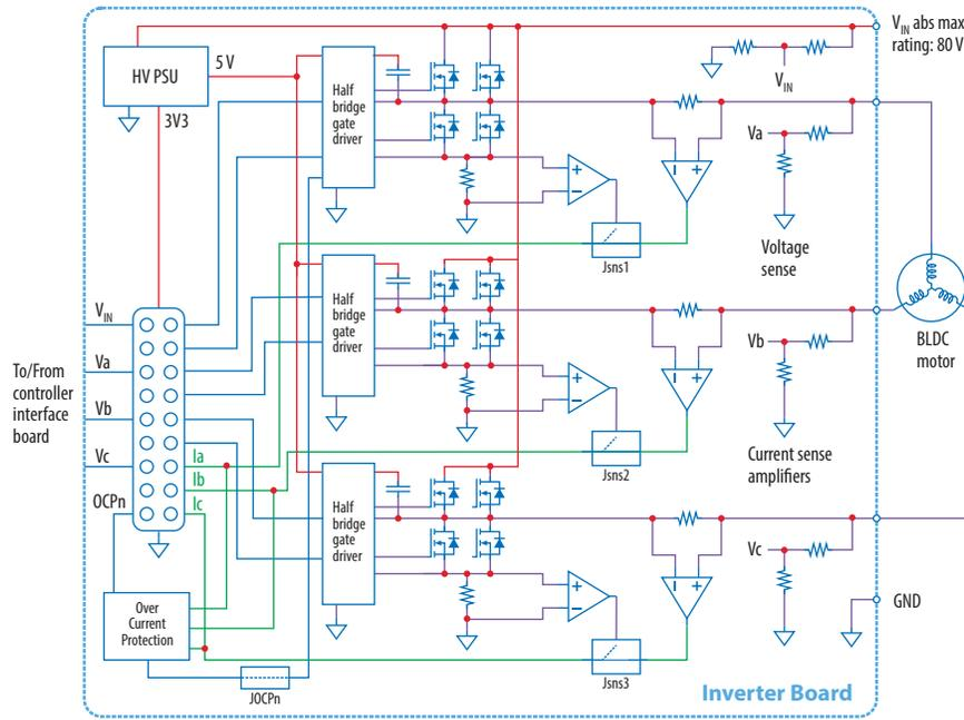
Figure 6. EPC9167 block diagram.
