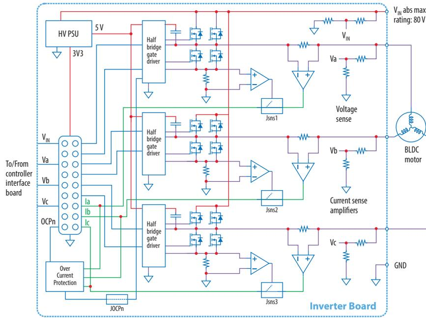
Figure 6. EPC9167 block diagram.
