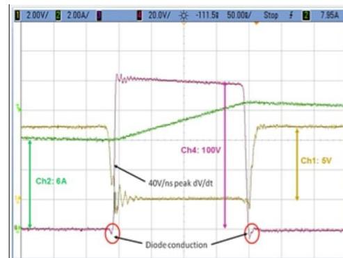
Figure 10: EPC1010 switching 100 V and 7 A using a discrete gate-drive solution. Ch1: low-side G-S voltage (2 V/div), CH2: inductor current (2 A/div), CH4: low-side D-S (switch-node) voltage (20 V/div). Time scale: 50 ns/div.
