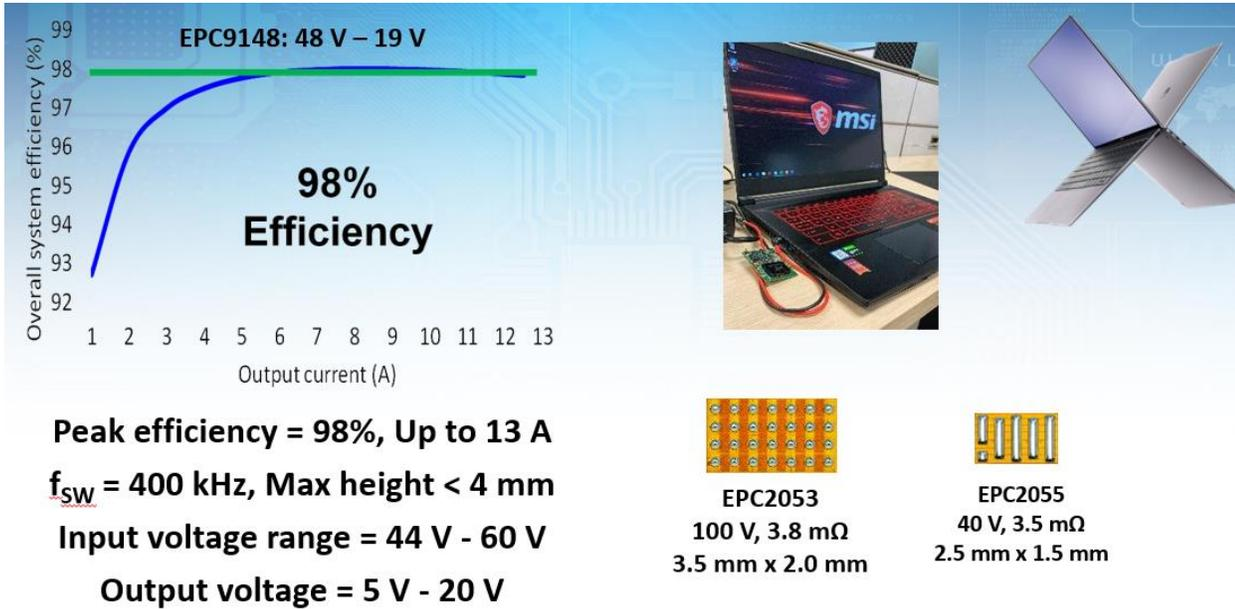
The EPC9148 reference design achieves its very high efficiency and low profile using one 100-V and three 40-V rated eGaN FETs.
