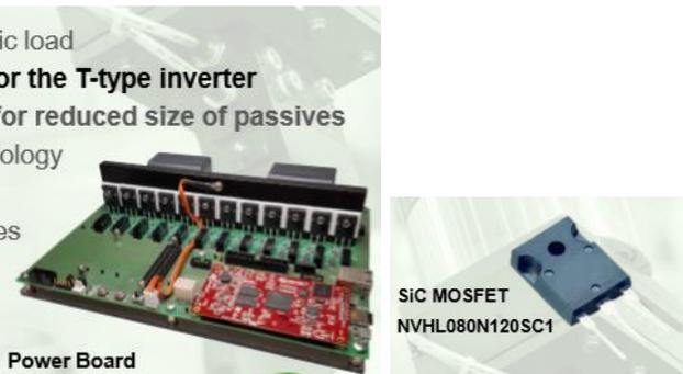
ON's T-type three-phase 10-kW inverter for motion control uses 80-m $\Omega$  NVHL080N120SC1 SiC MOSFETs.
