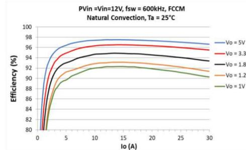
The IR3887M 30-A achieves high efficiency and small size using fast constant-on-time control.
