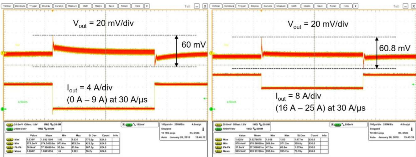
Load transient response of the IR3889 30-A iPOL. Pvin = 12 V, Vout = 1 V, fsw = 800 kHz, L = 150 nH, Cout = one 470-uF/2V + ten 22 uF + four 47 uF capacitors.
