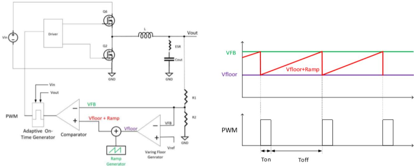
Infineon’s Fast COT control scheme adds a ramp signal with a varying voltage floor to generate its error signal to the PWM.
