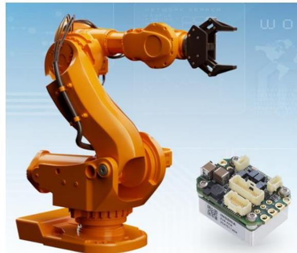
*Ingenia's Everest NET 30/80 servo drive designed for robotic and industrial applications uses eGaN FETs.*
