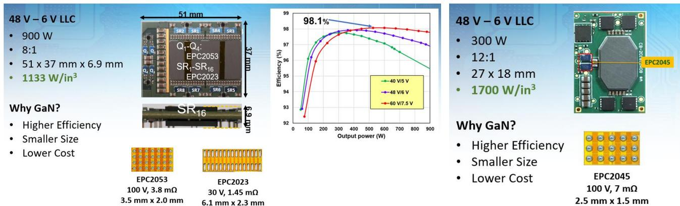
GaN-based LLC converters step down 48 V to 6 V with high power density.
