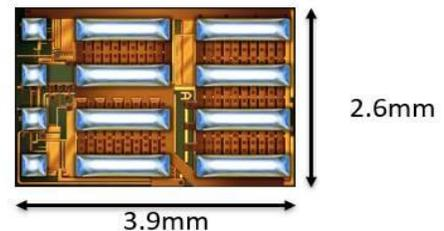
*EPC2152, a monolithic 80-V, 12.5-A half-bridge power stage IC with on-chip gate driver.*
