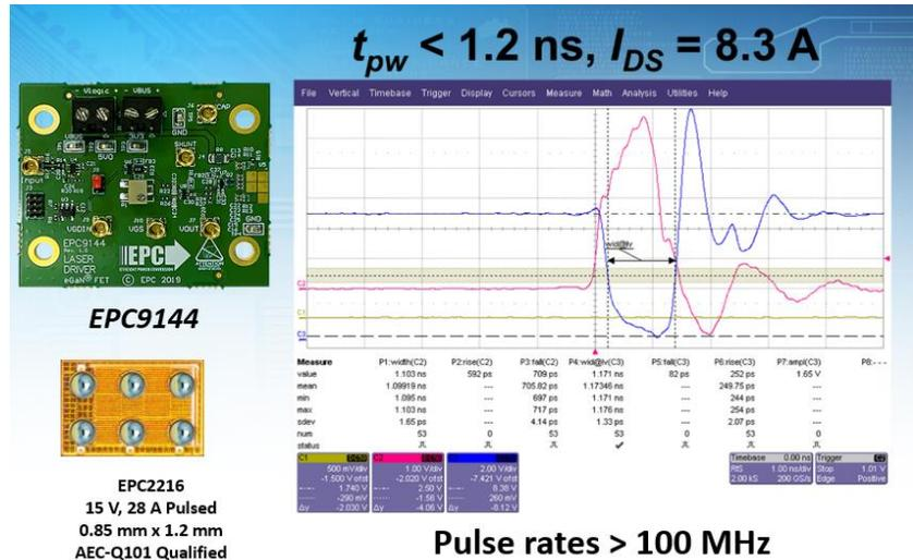
Using eGaN FETs to generate pulses for indirect time-of-flight LiDAR.
