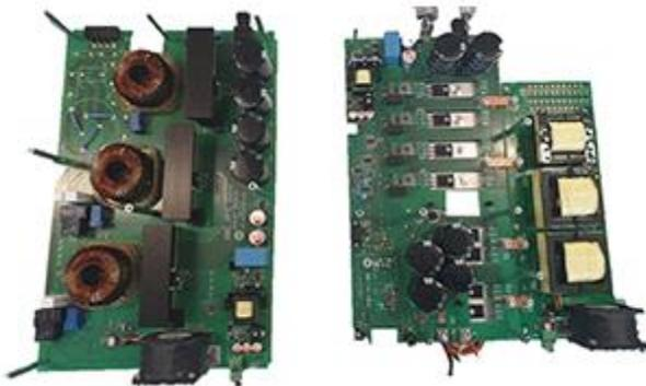
An 11-kW three-phase on-board charger from ON combines SiC-based PFC and LLC converter stages.
