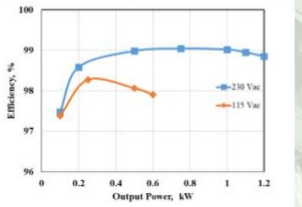
An 80 PLUS Titanium 1.2-kW TP-PFC board featuring ON's NTBG060N090SC1 SiC MOSFETs achieves 99% efficiency.
