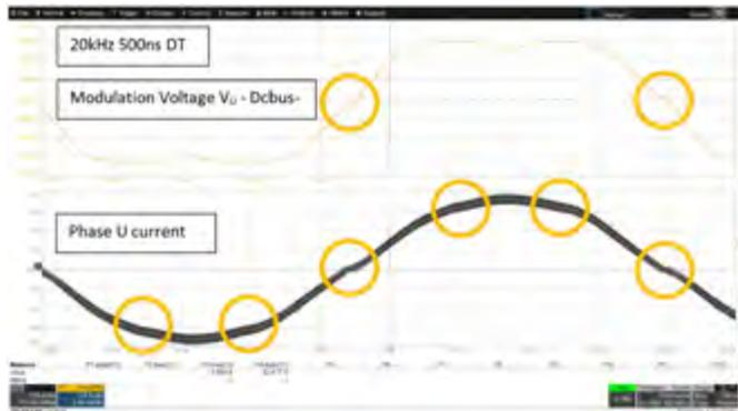
Figure 4a: Voltage modulation and phase current at 20 kHz with 500ns dead time
