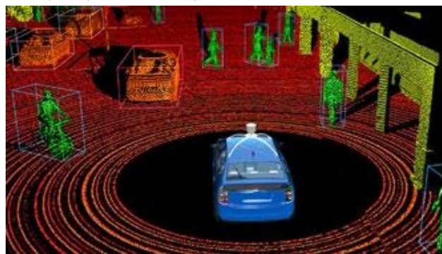
Figure 1: LiDAR sensors using GaN FETs create a fast and accurate digital point cloud that is used by autonomous cars to identify surrounding structures and obstacles.
