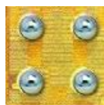
Figure 5: The 80 V EPC2203 device passed AEC-Q101 testing. It measures 0.9 x 0.9 mm and has a pulsed current rating of 18 A.
