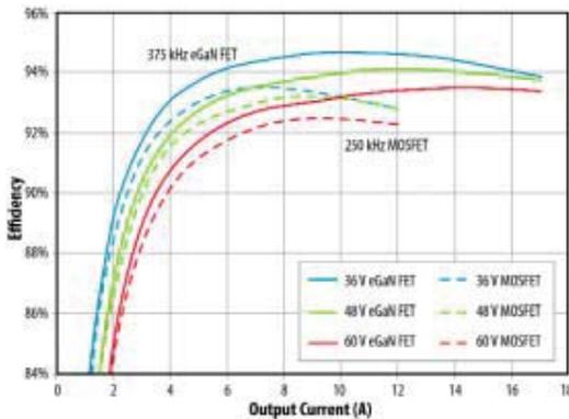
Figure 4: Efficiency comparison between eighth brick converters
