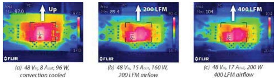
Figure 6: Thermal images of EPC9102 under different cooling conditions: (a) convection cooled, (b) 200 LFM, and (c) 400 LFM.
