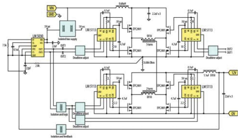
Figure 2: Block Diagram of EPC9102 Demonstration Board
