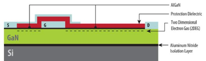
**Figure 1.** Simplified cross section of an eGaN FET
