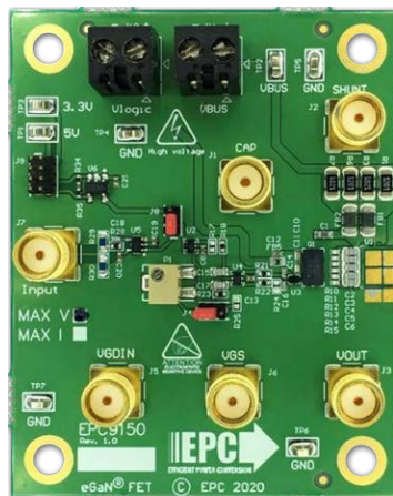
EPC9150 Long Range Lidar 221 A laser pulse peak 2.9 ns wide pulses
