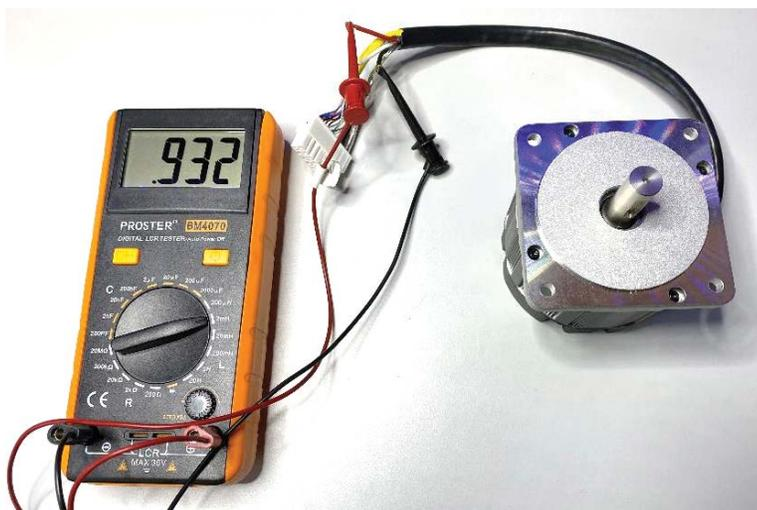
This motor has  $L_{L-L} = 932\text{ }\mu\text{H}$  line to line inductance (LCR meter leads may also have inductance, **use autozero function if available**)
