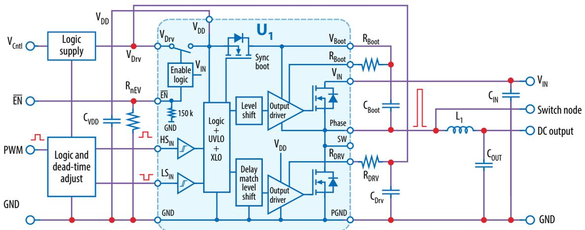
Figure 1: Block diagram of EPC90147 development board
