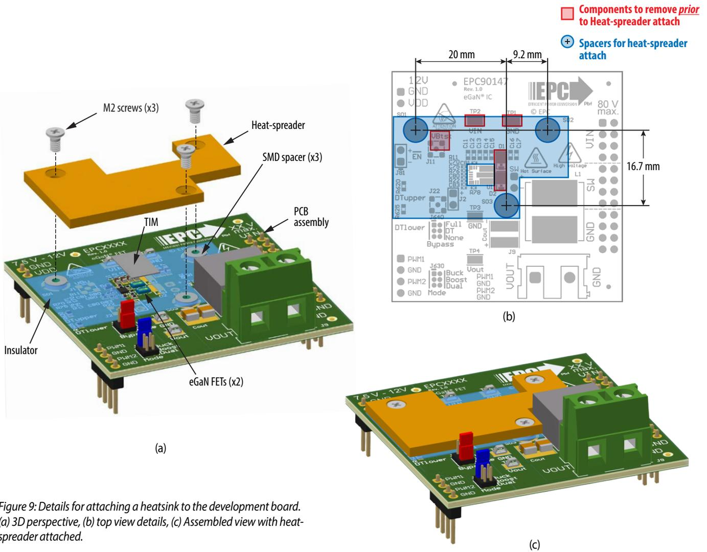
Figure 9: Details for attaching a heatsink to the development board. (a) 3D perspective, (b) top view details, (c) Assembled view with heat-spreader attached.
