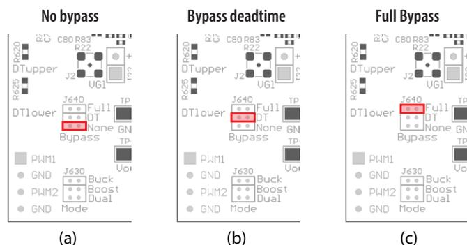
Figure 5: Bypass mode Jumper settings for J640
