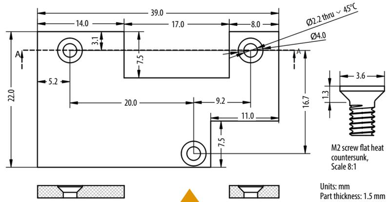
Figure 10: Heat-spreader details
