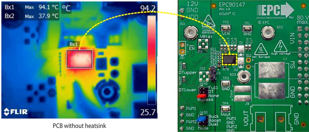
Figure 17: Measured thermal image showing the case temperature when operating under the following conditions:
