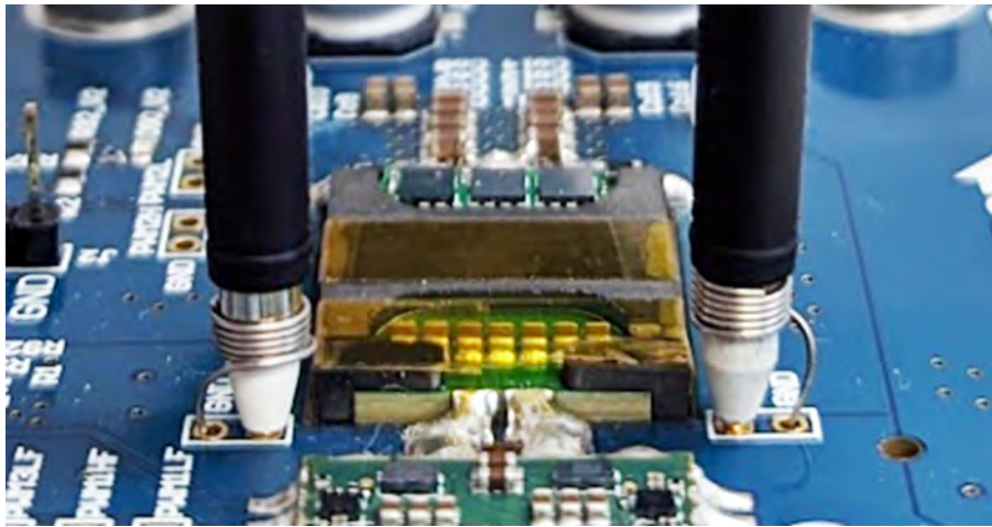
Figure 9: Recommended method for measuring switch-node voltages in the primary (SN1, SN2) and Drain voltages in the secondary (Vda, Vdb)
