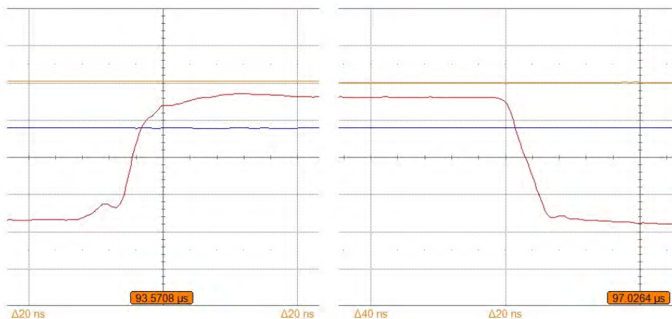
Figure 10 – Example waveforms at 20 A output, with zoom on switching node voltage edges.
