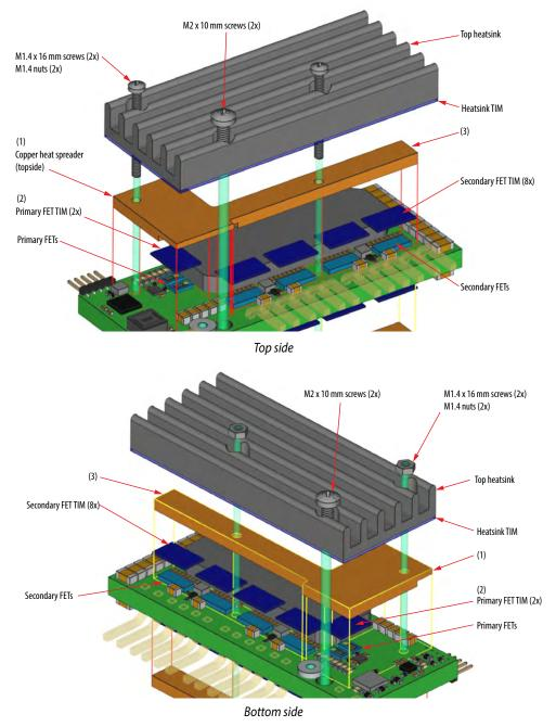
Figure 6: Thermal solution assembly process for the EPC9149 module
