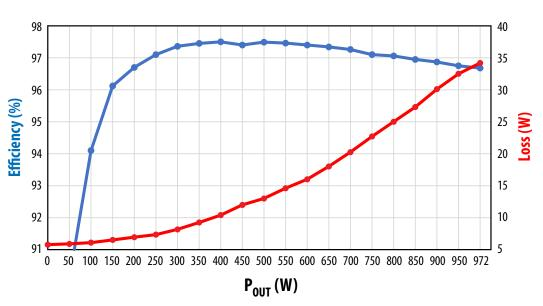
Figure 4: Total system efficiency and loss @ 12V output, 48V input voltage, 400LFM forced air cooling.
