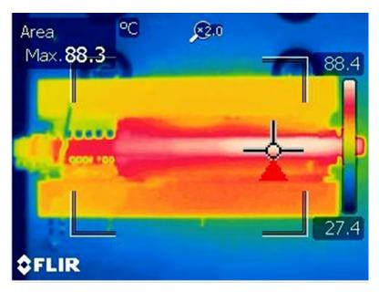
Figure 5: Thermal image of the EPC9149 operating at 48 V<sub>IN</sub>, 12 V and 83.3 A output, thermal steady state reached after 10 minutes, Top: primary FET junction temperature and Bottom: highest board temperature.
