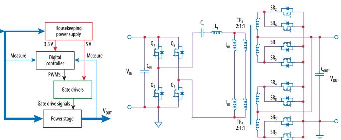
Figure 1: Simplified schematic diagram of the EPC9149 LLC Module
