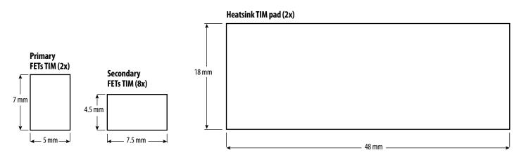
Figure 12: Drawings and dimensions of TIM pad cutouts for primary FETs, secondary FETs and heatsinks.
