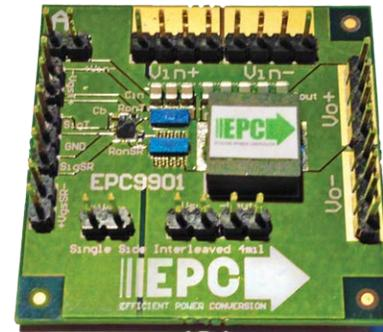
Figure 11: Experimental prototype for optimal design (Top Switch: EPC2015, Synchronous Rectifier: EPC2015, Driver: LM5113)
