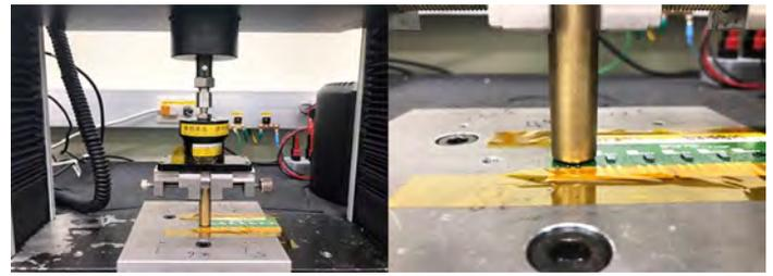
Figure 27: Pressure test instrument. The tester head lowers to the backside of the devices using a constant loading speed of 0.6 mm/min until the predetermined force is sensed by the gauge. The DUTs are surface mounted on a FR4 test coupon that is secured on the testing stage.
