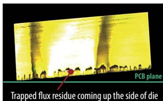
Figure 3: Tilted die trapping residual solder flux.
