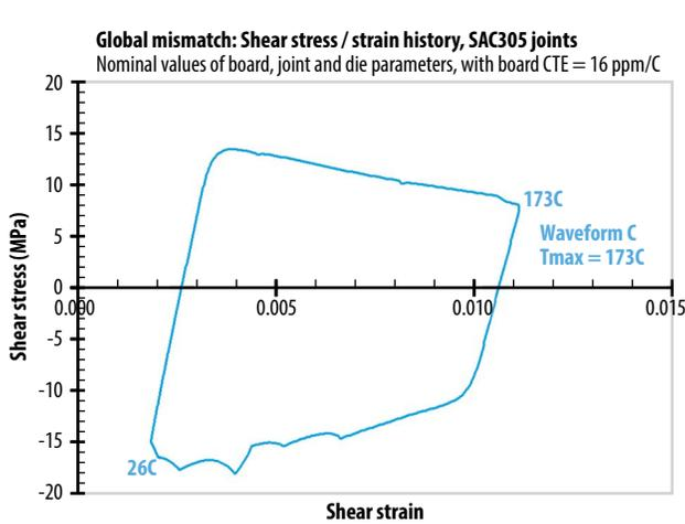
Figure 12. Calculated solder joint strain energy density during IOL cycle  $\Delta T_j = 150^\circ\text{C}$  (EPC80xx: 2.05 mm x 0.85 mm).
