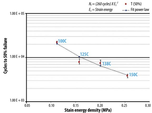
Figure 13. IOL thermal model: number of cycles to failure versus solder joint strain energy density (error bars represent 67% confidence).
