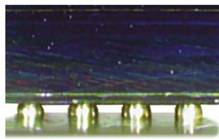
Figure 4: Properly mounted device.
