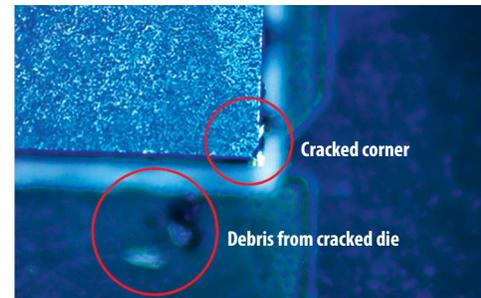
Figure 5: eGaN® Field failure showing die corner chipping caused by inadequate clearance of pick and place tool while placing components adjacent to the eGaN® FET.
