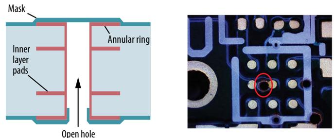
Figure 6: (a) Diagram of via with solder mask tent covering. (b) PCB showing uncovered via.
