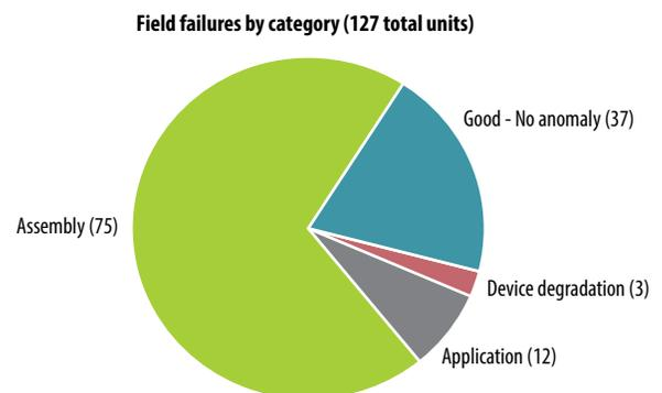
Figure 1: Field failure breakdown by root cause category.
