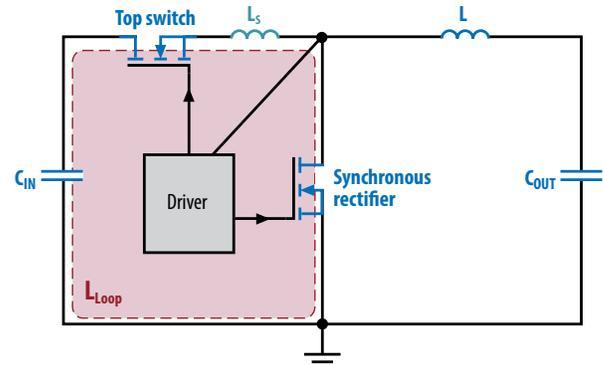
Figure 7: Synchronous rectifier showing parasitic inductances ( $L_S$  is common source inductance) ( $L_{Loop}$  is high frequency power loop inductance) ( $L_{Loop}$  is high frequency power loop inductance)
