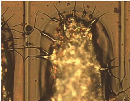
Figure 2: eGaN® FET showing dendrite formation due to residual flux.
