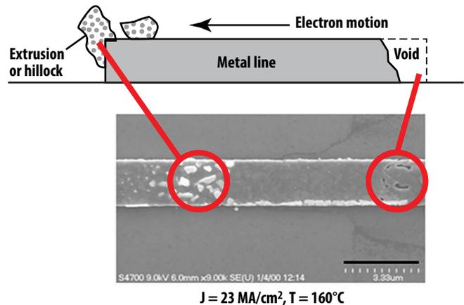
Figure 10: Effects of electromigration on a metal conductor via scanning electron microscope: voids and atom accumulation observed [from 18].
