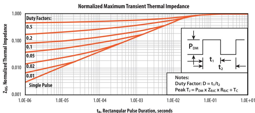
Figure 1. Normalized transient thermal impedance  $Z_{\theta JC}$
