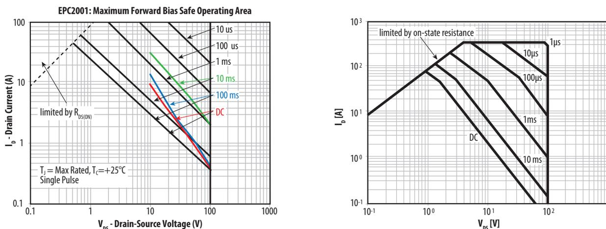
Figure 3. EPC2001 (left) and BSB056N10NN3 (right) Safe Operating Area
