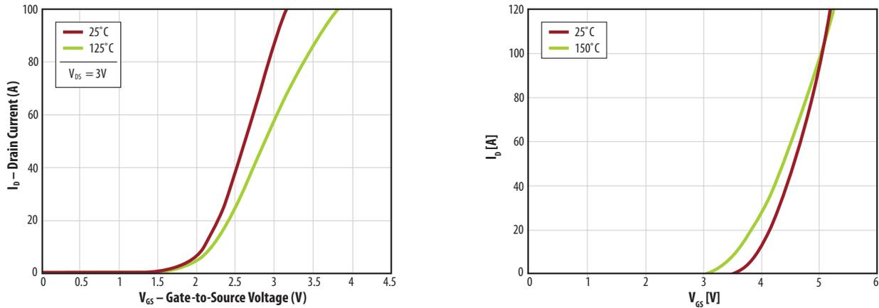
Figure 2. EPC2001 (left) and BSB056N10NN3 (right) transfer characteristics
