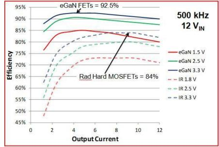
Fig. 3. Buck converters using radiation hardened eGaN FETs offer much higher efficiency compared to rad hard silicon MOSFETs.
