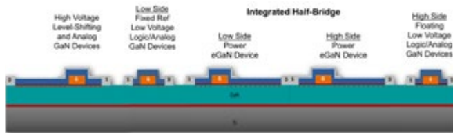
Figure 5: Cross section of a monolithic power stage showing high-side and low-side power devices with their accompanying low voltage driver and level shift devices
