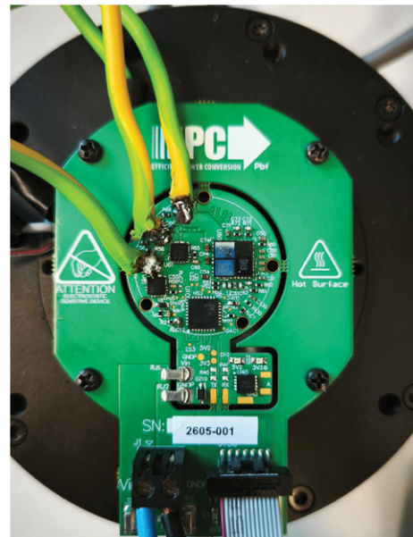
Figure 5a: EPC91132 with outer PCB ring mounted in a humanoid joint motor
