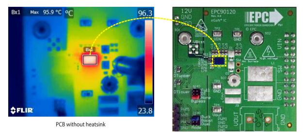
Figure 16: Measured thermal image showing the case temperature when operating under the following conditions:  $f_S = 1 \text{ MHz}$ ,  $I_{OUT} = 10 \text{ A output}$ , 25°C ambient and high airflow
