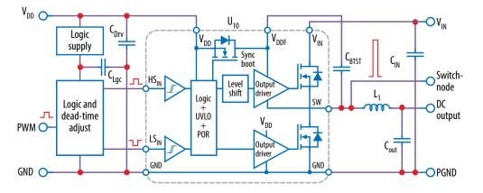
Figure 1: Block diagram of EPC90120 development board
