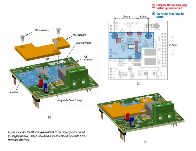
The design of the heat-spreader is shown in figure 11 and can be made using **aluminum** or **tellurium copper** for higher performance.
