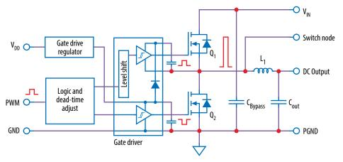
Figure 1: Block diagram of EPC90154 development board default configuration
