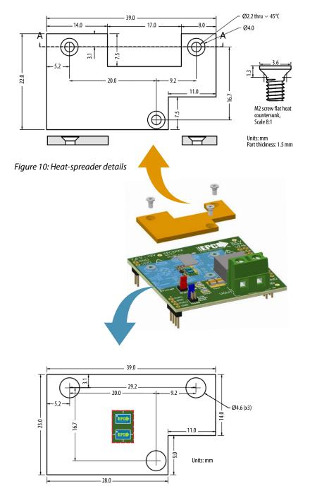
Figure 11: Insulator sheet details with opening for the TIM with location of the FETs
