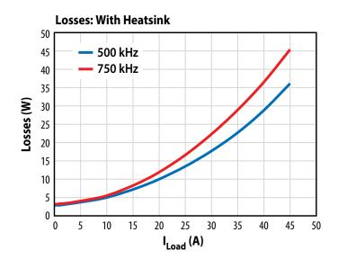
Figure 15: Measured efficiency and power loss operating at various switching frequencies and using  $L = 2.2 \mu H$
