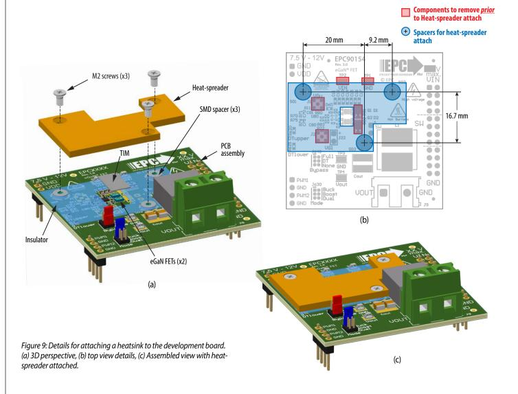
The design of the heat-spreader is shown in figure 10 and can be made using **aluminum** or **tellurium copper** for higher performance.
