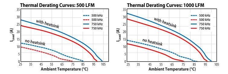
Figure 17: Typical thermal derating curve for two air flow rates, with and without a heatsink attached, measured with the board operating at various switching frequencies and using a 2.2 µH inductor
