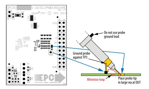
Figure 3: Proper measurement of switch node – OUT.
