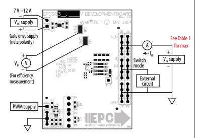
Figure 2: Proper connection and measurement setup.
