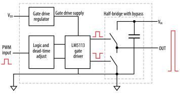
Figure 1: Block diagram of development board.
