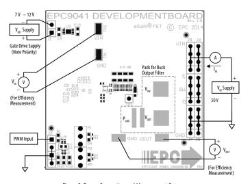
Figure 2: Proper Connection and Measurement Setup
