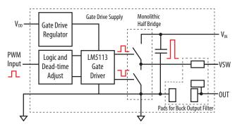
Figure 1: Block Diagram of Development Board
