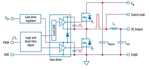
Figure 1: Block diagram of EPC9097 development board
