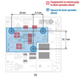
Figure 10: Details for attaching a heatsink to the EPC9097 board.
