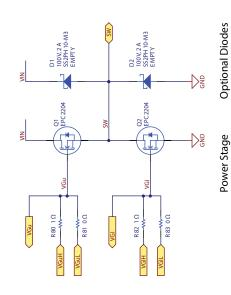
Figure 12: EPC9097 Power Stage schematic
