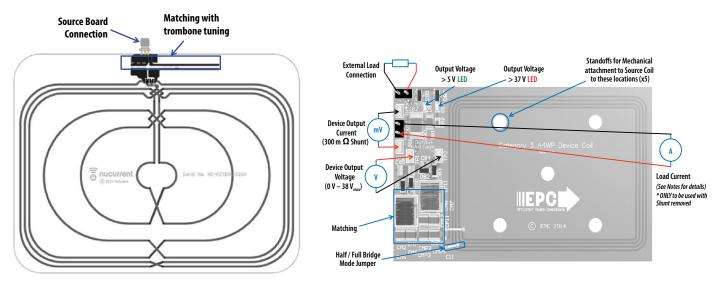
Figure 6: Proper Connection for the Source Coil
