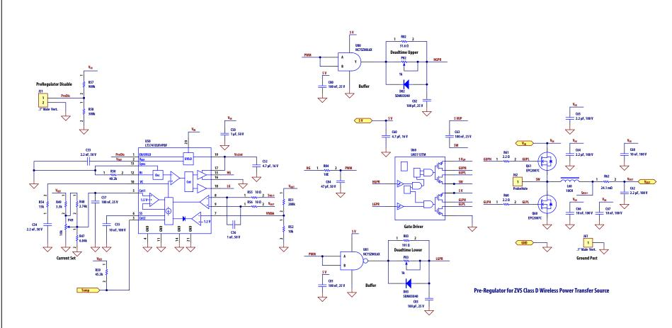
Figure 21: Pre-Regulator for ZVS Class D Wireless Power Transfer Source
