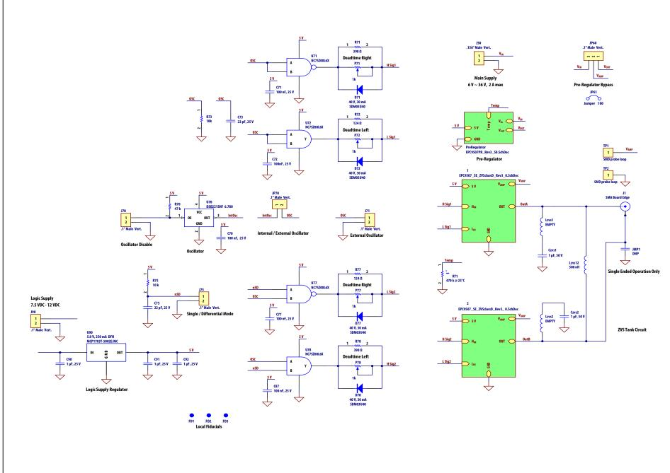
Figure 10: Differential ZVS Class D Wireless Power Source Board using EPC2014C
